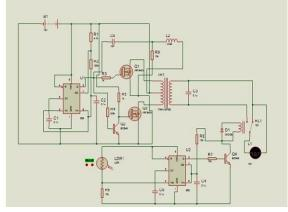
Fig: 2. Circuit Diagram of Single Phase Series Resonant Inverter
